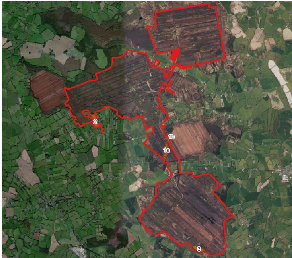
Figure 3-8 Proposed Borrow Pit Locations. Location 1a and 1b in Carranstown Bog (selected), Location 2 in third party land (selected), Location 3 Ballivor Bog (not selected)
